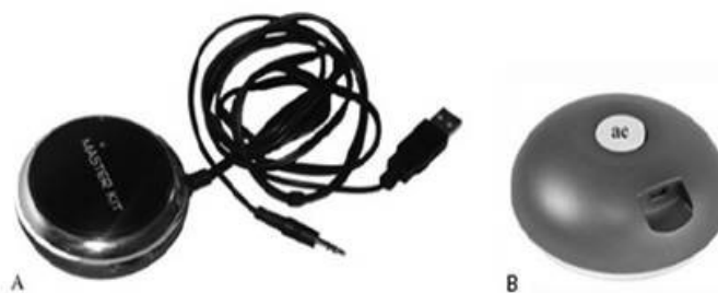
Rice. 3. Vibrodynamic MT6030. Pos. "A" - general view; Pos. "B" - bottom view. Letter combination "ae" the active element vibrodynamics is marked.
