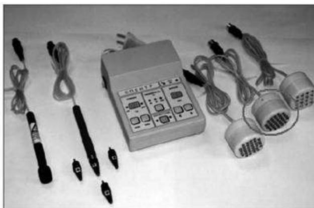
Rice. 1. Apparatus physical therapy Spectrum LC-02. Oval marks the matrix of green LEDs, which was used in this work.
